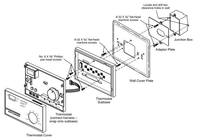
Figure 11. Mounting 1F62 thermostat to vertical junction box
